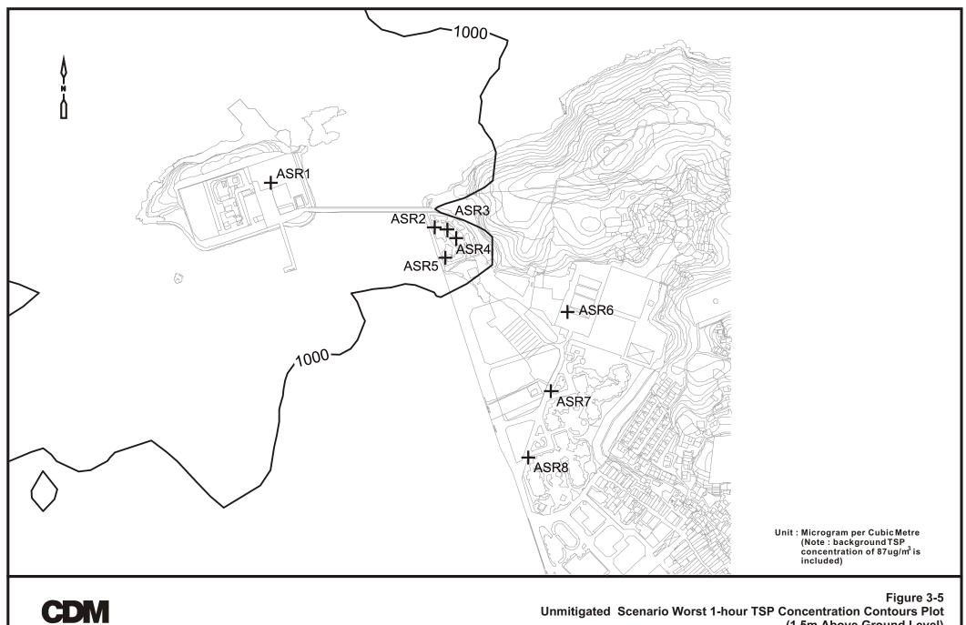
Figure 3-5 Unmitigated Scenario Worst 1-hour TSP Concentration Contours Plot (1.5m Above Ground Level)
